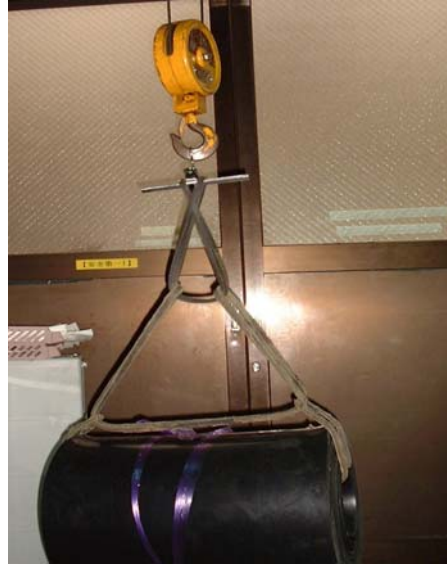
U.H.N pull by tension testing (Load 50kg)
